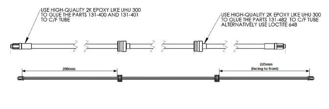
GLUE MA131-400 WITH MA131-401 AND TOGETHER TO C/F TUBE
