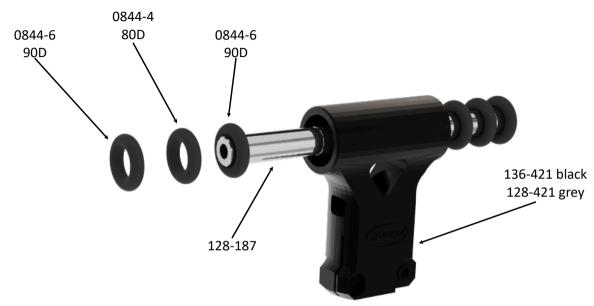
Assembly Tip: Apply some grease, vaseline or tallow to the o-rings and to the spindle shaft. The picture above shows a typical setup for dampening. If you do sport flying you can use two or three 80D o-rings on each side also.
