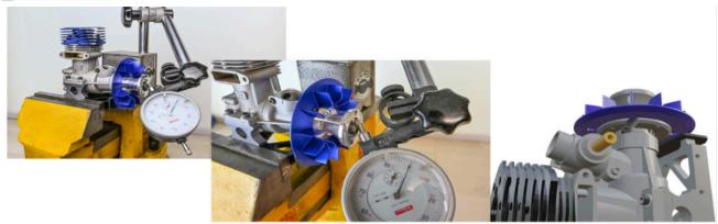
INSTALLING THE PREPARED FAN HUB: TO INSTALL THE FAN HUB YOU SHOULD USE A CRANKSHAFT LOCKING TOOL. TO USE IT YOU HAVE TO REMOVE THE BACK PLATE OF THE ENGINE. TAKE CARE ABOUT THE ORIENTATION AND CORRECT USE OF THE TOOL (SEE ENGINE MANUAL). OHTERWISE YOU CAN DAMAGE THE PISTON / ENGINE. DO NOT USE A PISTON STOPPER WHICH IS INSTALLED AT THE GLOW PLUG BORE.
