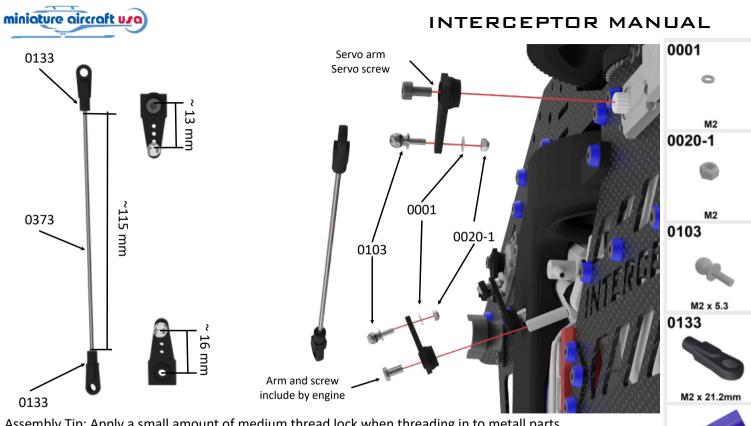
Assembly Tip: Apply a small amount of medium thread lock when threading in to metall parts.
