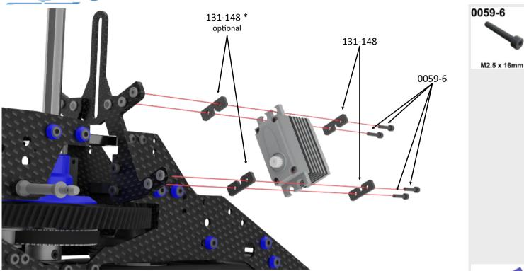
\* MA131-148 Servo Spacers are included. Add for proper servo linkage alignment, if required.
