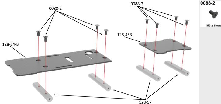
Apply a small amount of medium thread lock when threading in to metall parts.
