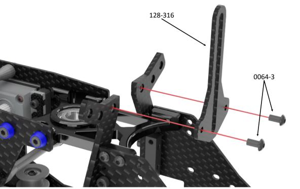
Assembly Tip: Apply a small amount of medium thread lock when threading in to metall parts.
