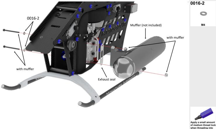
Apply a small amount of medium thread lock when threading into metal parts.
