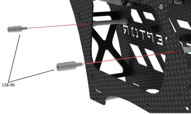
Assembly Tip: Apply a small amount of medium thread lock when threading in to metall parts.
