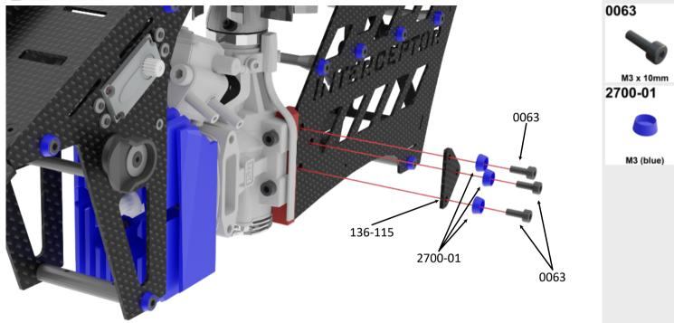
Assembly Tip: Do not completely tighten the bolts 0063 at this assembly step. The engine shall be still moveable forward and backward.
