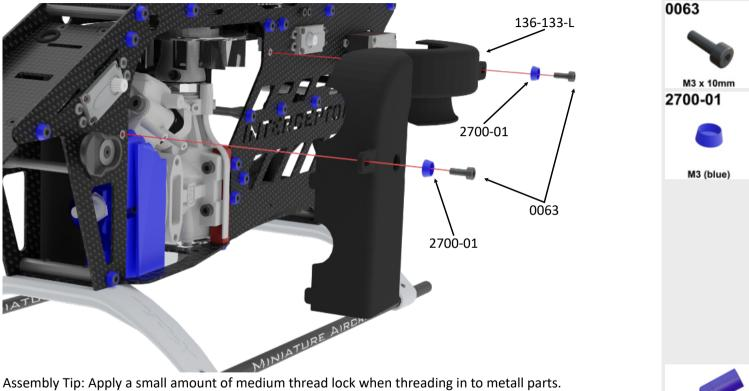
Check that fan shroud left and right fit together.
