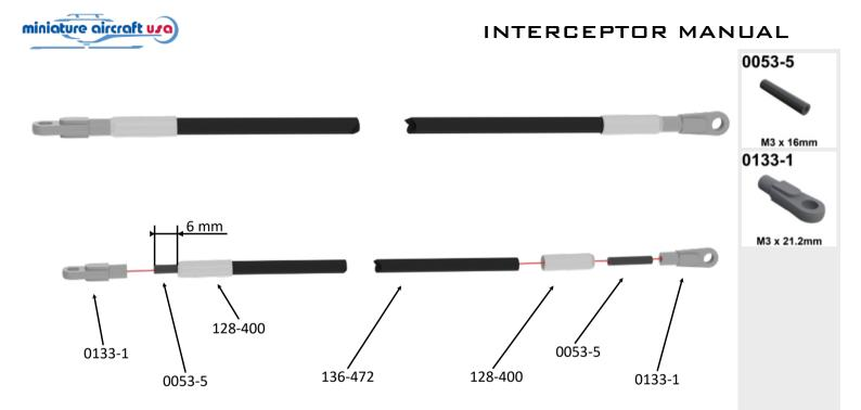
Assembly Tip: Put all parts together and check length of the push rod. Shorten carbon tube if nescessary. Install the 0053-5 set screws into the push rod ends using high quality epoxy. Use high quality epoxy to glue the push rod ends to the carbon tube. Put epoxy at the inside and the outside of the carbon tube to glue the push rod ends on it.
