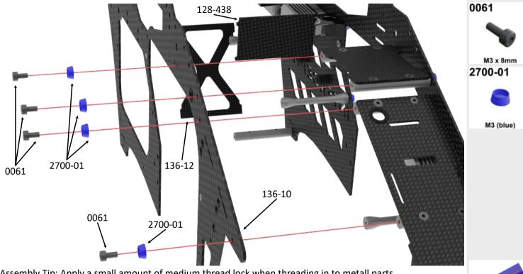
Assembly Tip: Apply a small amount of medium thread lock when threading in to metall parts.
