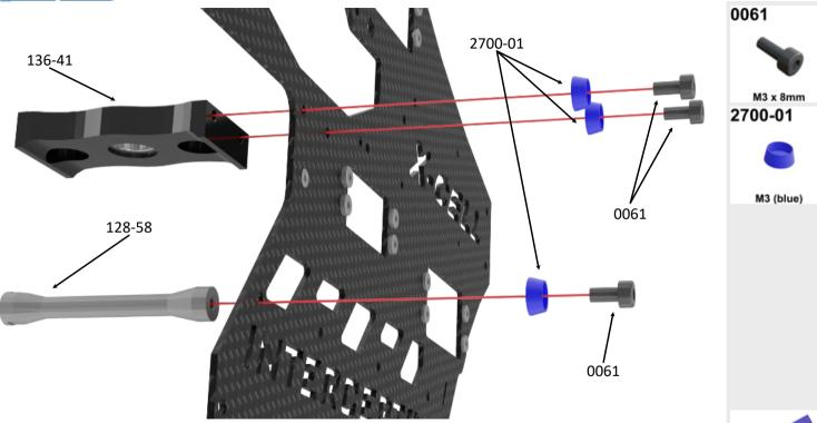
Apply a small amount of medium thread lock when threading in to metall parts. For this assembly step put the mainshaft into both bearing blocks temporarily to ensure that the bearing blocks are aligned well.
