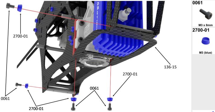
Assembly Tip: Do not completely tighten the bolts 0061 at this assembly step. The engine shall be still moveable forward / backward and up / down. Move the engine up til the clutch and clutchbell align. Tighten the bolts 0081. Turn the startshaft clockwise and move the engine forward/backward until the startshaft can be turned easy without force. Try to find the optiaml position. Then tigthen Bolts 0061 and 0063.
