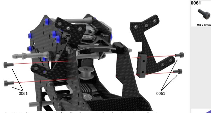
Assembly Tip: Apply a small amount of medium thread lock when threading in to metall parts.
