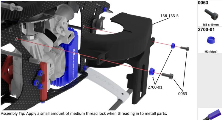
Check that fan shroud left and right fit together.
