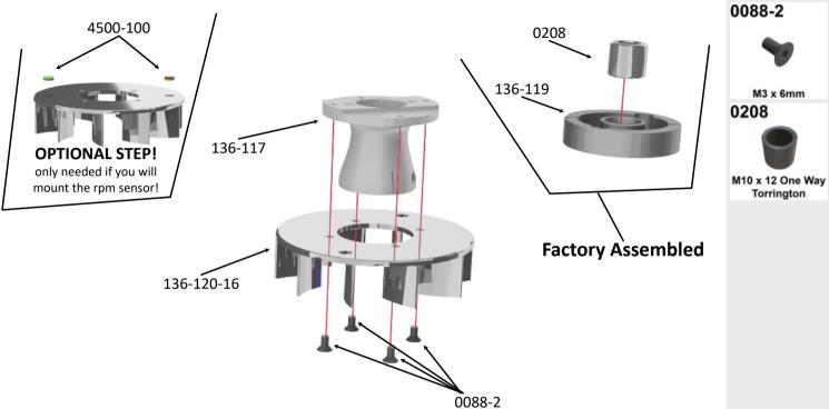
If using a governor sensor install the magnets at the fan. Take care of the orientation. On shall be facing up "North" the other shall be facing up "South". Use some high quality two-component epoxy like UHU 300 and let it harden. The magnets are included in the Interceptor kit. Always install both magnets to ensure a well balancing.
