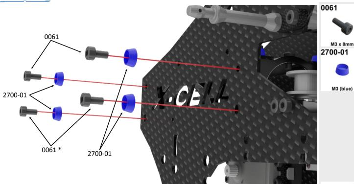
\* NOTE: 0061 BOLTS ARE NOT TIGHT AT THIS TIME. Remove later to install boom if necessary.
