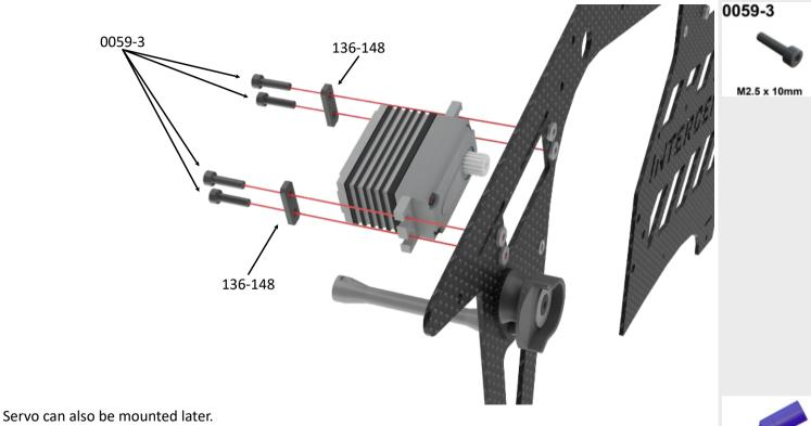
Apply a small amount of medium thread lock when threading into metal parts.
