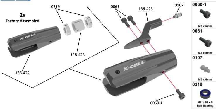
Assembly Tip: Take care about the orientation of part 128-425. Compare its orientation to fit part 136-422. First time Factory Assembled.
