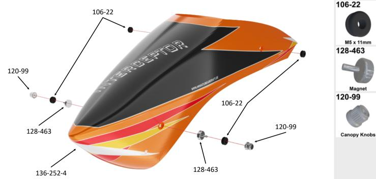
Assembly Tip: Apply a small amount of medium thread lock when threading in to metall parts.
