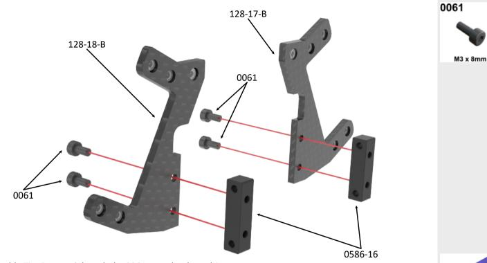
Assembly Tip: Do not tighten bolts 0061 completely at this step. After installing part 128-316 check alignment of all parts and then tighten all bolts.
