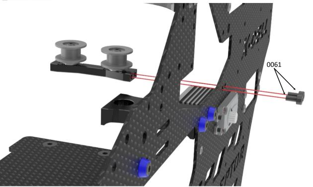
Assembly Tip: Align the belt idler mount that the belt idlers are parallel to the main shaft.
