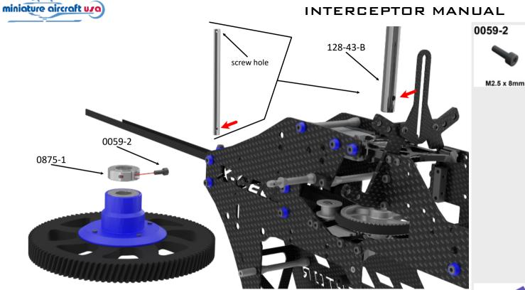
Assembly Tip: put a small amount of synthetic grease into the one way bearings of part 136-450 before installing the main shaft. Take care about the orientation of the main shaft. The through hole faces to the top of the helicopter.
