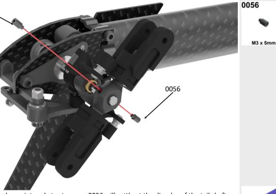
Assembly Tip: Take care that the dog point socket set screws 0056 will settle at the dimples of the tail shaft. First install the screws that they settle correctly at the dimples but do not tighten them. Then tighten one of bolts firmly and then the other one slightly less.
