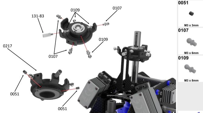
Thread in the MA0051 m3x3 socket set screws into the bottom ring of the swashplate until they touch the lower bearing. They are used to apply slight pressure on the bearing to adjust bearing play if needed. If too much pressure is applied with the MA0051 m3x3 socket set screws, the bearing will fail.
