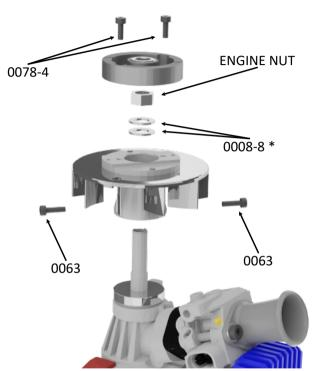
Use crankshaft clamp tool O.S. 71530530 to hold crankshaft while tightening.
