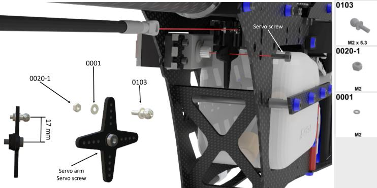
Assembly Tip: Read servo manual for installing servo screw
