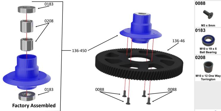
Assembly Tip: Apply a small amount of medium thread lock when threading in to metall parts.
