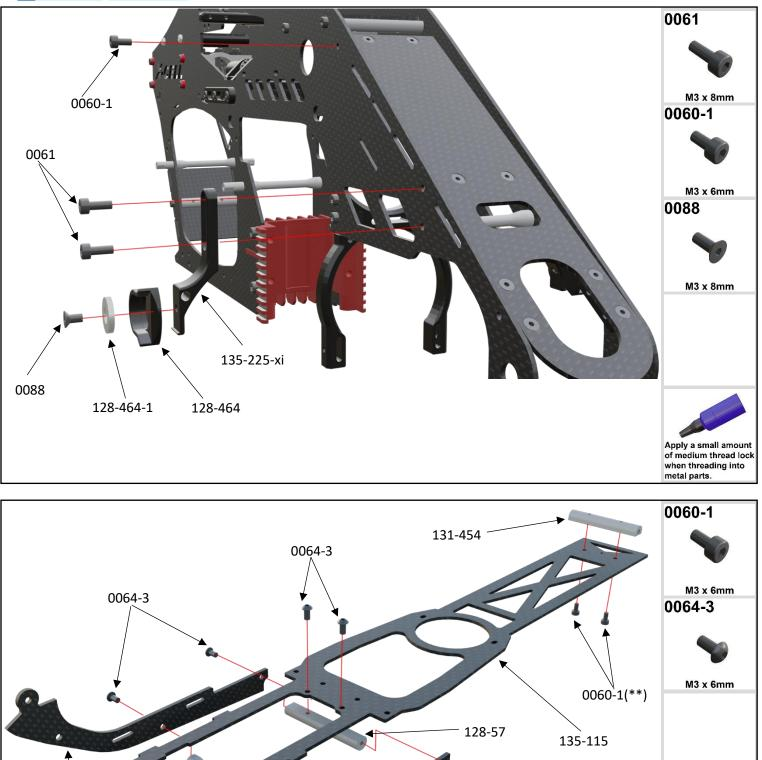
Do not supply thread lock at screws marked with a (\*\*) at this assembly step. They will be removed again later.
