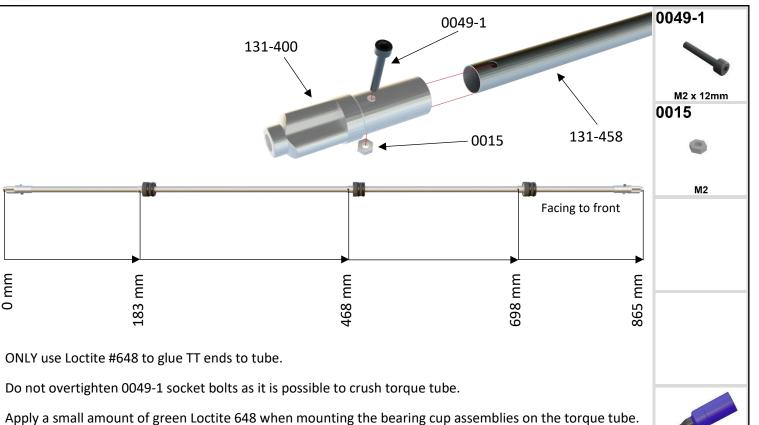
NOTE: Carefully glue bearing assemblies to torque tube making sure bearing locations are NOT equal distances from torque tub ends. Allow Loctite 648 to dry (about 2 hours) before installing into tail boom.
