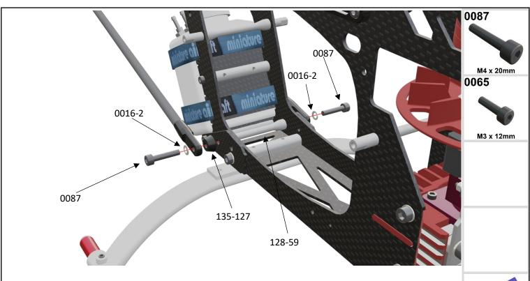
In this step tighten the screws from the rear Boom Support Mount and the Support ends. The use of thread lock MA3200-20 (loctite #243) is recommended on MA0078 Socket Bolts.
