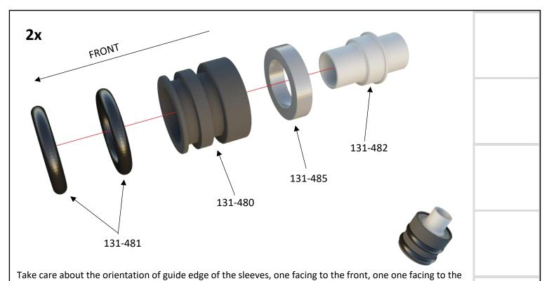
Apply a small amount of green Loctite 648 when mounting the bearing cup assemblies on the torque tube.
