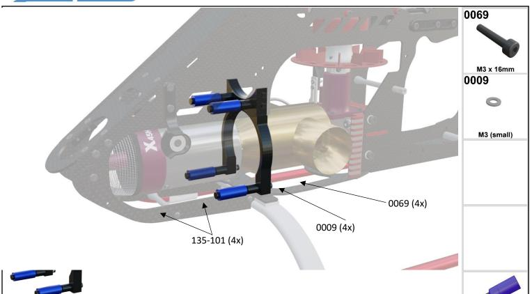
Install turbine supports (135-101). The supports shall only 'touch' the engine. They shall not supply pressure to the engine body.
