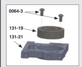
Middle Main Shaft **Bearing Block** (Factory Assembled)
