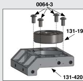
NOTE: Middle bearing block features threaded holes.
