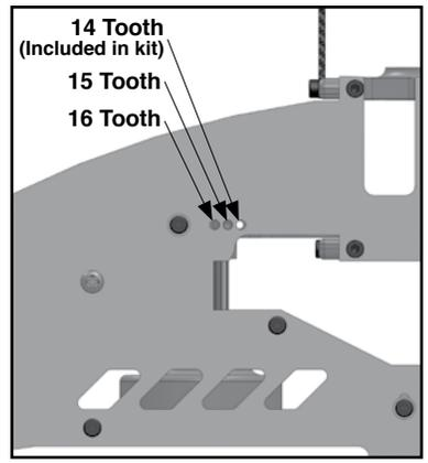
NOTE: Motor Mount and Lower Pinion Bearing Block bolt locations for proper gear mesh.
