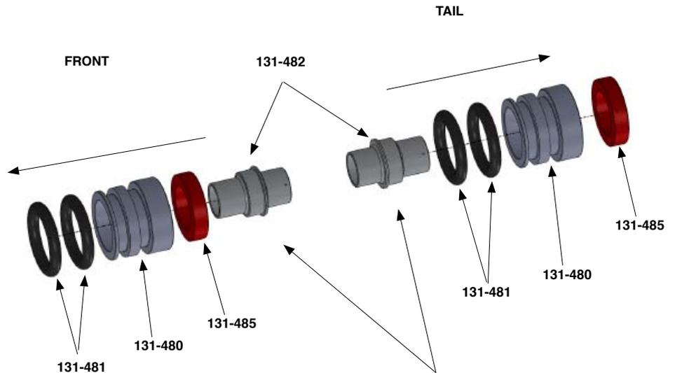
Take care about the orientation of guide edge of the sleeves, one facing to the front, one one facing to the tail.
